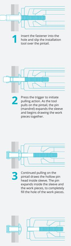
A solid circle lock between the pin and sleeve is formed just prior to the pin breaking flush with the sleeve head, completing the installation.
